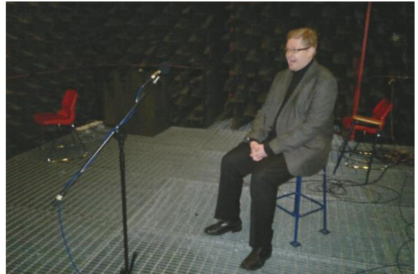
Test person screaming in an anechoic chamber
